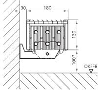
Diag. 10 Section through wall-mounted unit
