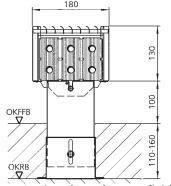
Diag. 7 Section through an unfinished floor unit.
