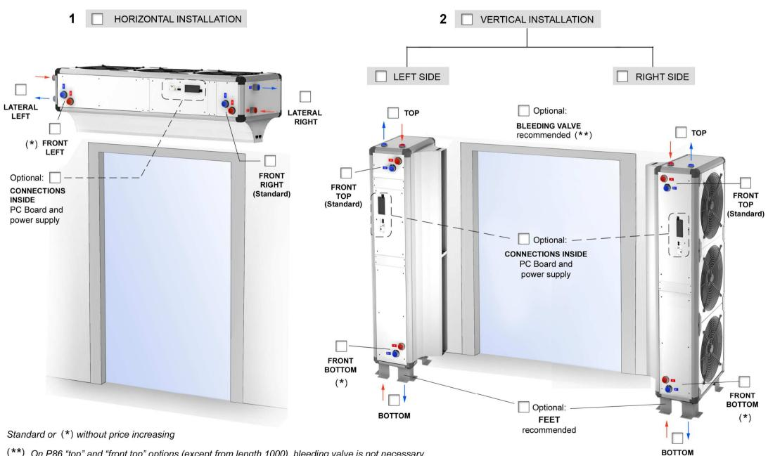
(\*\*) On P86 "top" and "front top" options (except from length 1000), bleeding valve is not necessary. In all other coils and options in vertical installation, bleeding valve is recommended in order to achieve the maximum power heating avoiding air inside the coil.
