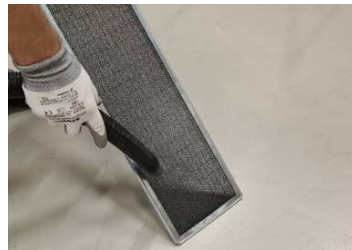
Vacuum the filter and re-fit it after cleaning.
